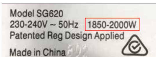
Example electrical appliance label, with input watts highlighted in red.
